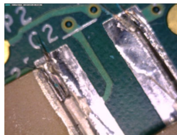
Board 4, C1 flux on cap underside, no visual residue on PCB
