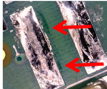
Board 1, C2 flux on cap underside and on PCB
