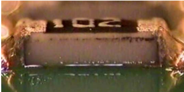
Figure 1: Flux residue trapped under component
