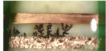
Figure 5 Dendritic Growth between 2 terminals underneath electronics
